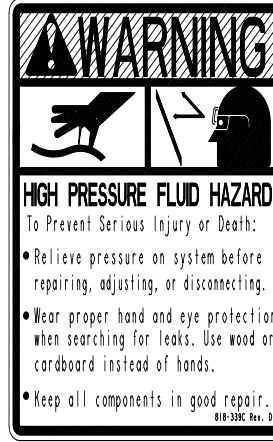
818-339C Warning - High Pressure Fluid Hazard
